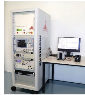
Rackmount system Includig CS114
